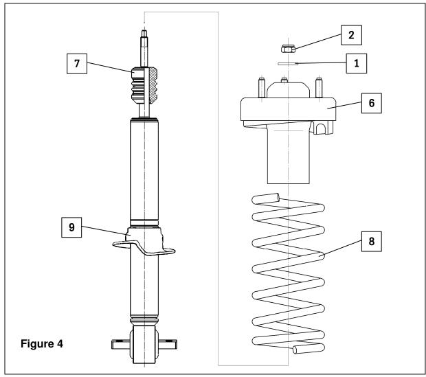
L. Install assembly on to the vehicle and tighten all fasteners to vehicle manufacturer's specifications. This completes the installation.
