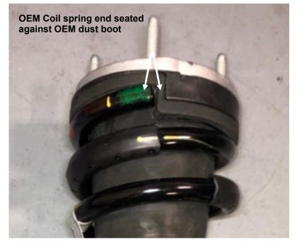
Figure 4: OEM Coil spring clocking
