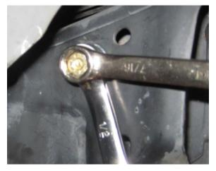
N. Remove the screw, washer, and flange nut. The Threaded Insert should now be rigidly fixed in the hole as shown below.
