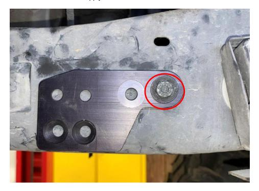
S. Remove the Reservoir Bracket (BOM item #1) and drill a 25/64" (10mm) hole at the marked locations. Install the ¼-20 Threaded Inserts (BOM item #9) provided into those holes. Refer to step K-N on how to install them. Apply for both sides.
