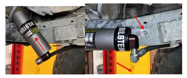
X. Position the reservoirs on both sides as shown and confirm it is not contacting anything on the vehicle. Tighten the Socket Head Cap Screw (BOM item #4) to secure the reservoir in place. Torque the Socket Head Cap Screw to 6 ft-lb (8 Nm). Repeat for the other side.
