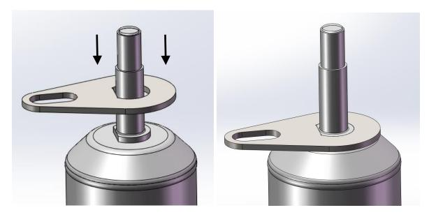
E. Slide the Lower Bushing (BOM item #14) and the appropriate Alignment Washer for your vehicle (BOM item #16 or #19 depending on year; see BOM on page 2) over the threaded pin on the shock body as shown below.
