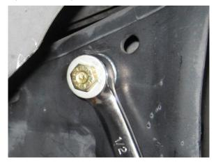
M. While keeping the Threaded Insert flange firm and parallel against the frame rail, tighten the hex head cap screw (BOM item #6) using a 7/16" box end wrench or socket. Turn it 2.5 rotations to set the Threaded Insert. Tightening in ¼ turn increments tends to work well.
