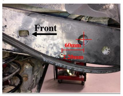
Drill 25/64" (10mm) hole and install threaded insert
