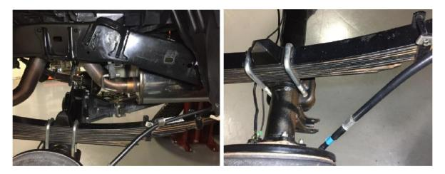
**B.** Carefully slide the reservoir bracket (BOM item #1) over the reservoir as shown below. Apply nonpermanent thread locker to the M6x1 socket head cap screw (BOM item #5) and slide it through the counter-bored hole in the reservoir bracket. Thread the socket head cap screw in enough so it won't fall out, but loose enough so you can still slide the reservoir in the bracket for adjustment.
