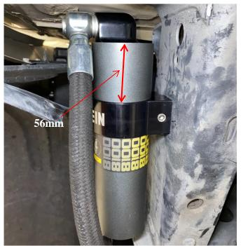
J. With the reservoir now secured to the chassis, rotate the right (passenger) side working tube so the hose swivel is clocked towards the front of the vehicle. For the left (driver) side, rotate the working tube so the hose swivel is clocked towards the back of the vehicle. On both sides, the working tube should be clocked until there is approximately 6mm (1/4") clearance between the hose swivel and the chassis shock tower. This is needed to ensure clearance with the tire.
