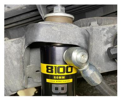
E. Align the lower shock mount in the rear axle attachment point using the OE lower shock bolt that was removed in step A (1 per side). Make sure the hex head of the bolt is facing the outside of the vehicle. Install the lower mount the same way it was removed and tighten the OE flange nut until the gap between the components and the rear axle attachment point is taken up as shown below. Do not torque the bolt and flange nut at this time. (The lower shock mount should still be free to rotate.)
