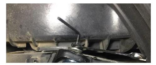
L. Fully tighten the lower shock bolt to the torque specified in the manufactures service manual.
