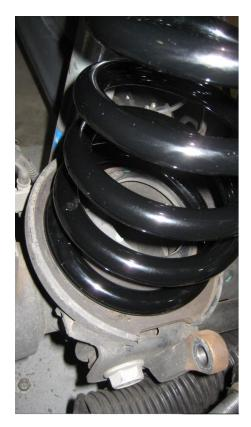
Figure 5. Passenger side (pictured with Bilstein **5100** shocks)
