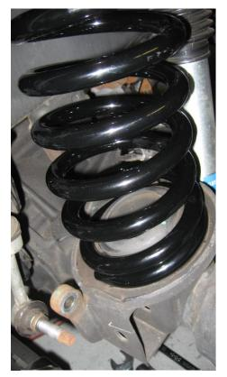
Figure 7. Driver side (pictured with Bilstein 5100 shocks)
