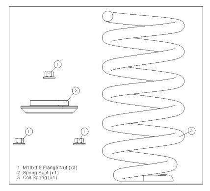
Fig 3: Bilstein supplied components
