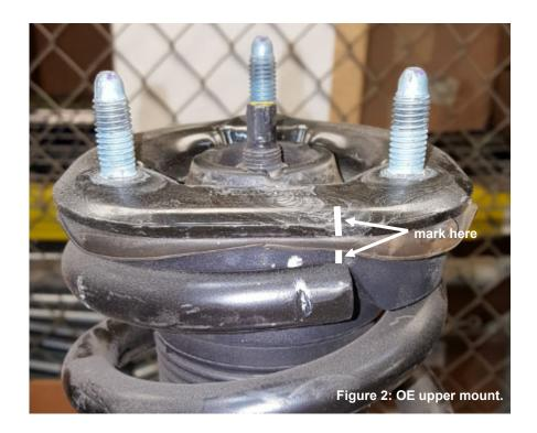
D. Using an appropriate spring compressor, compress the spring until it can be rotated freely by hand. Then, disassemble the shock and spring unit.
