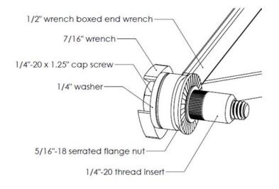
Figure 3: Threaded Insert, Hand Tightened
