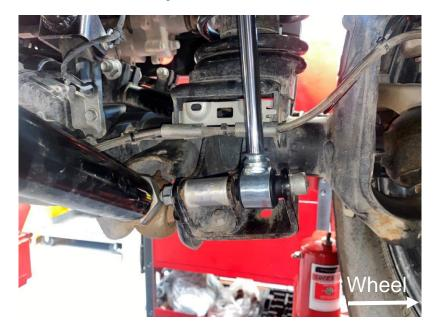
Figure 14: Passenger Side Bottom Mount
