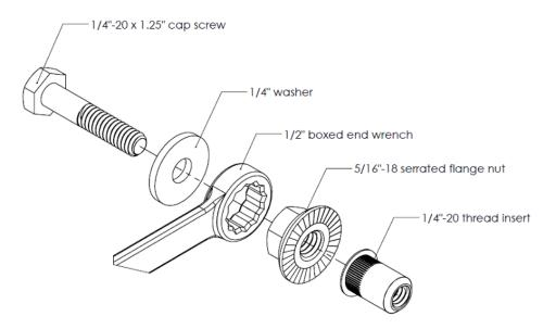
Figure 2: Threaded Insert, Parts/Tools Required
