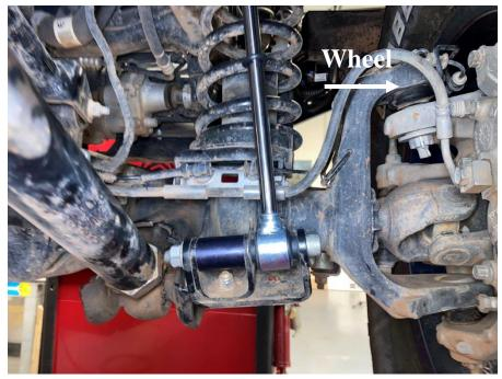
Figure 13 – Passenger side bottom mount
