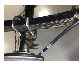
B. Carefully slide the reservoir bracket (BOM item #1) over the reservoir as shown below. Apply non-permanent thread locker to the M6x1 socket head cap screw (BOM item #5) and slide it through the counter-bored hole in the reservoir bracket. Thread the socket head cap screw in enough so it won't fall out, but loose enough so you can still slide the reservoir in the bracket for adjustment.
