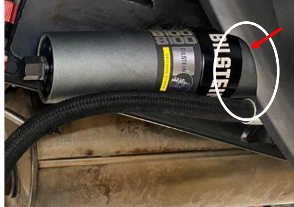
Inner fender liner clearance
