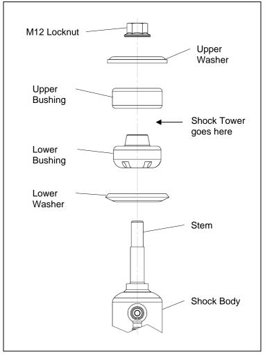
Figure 2. Shock Mount Assembly
